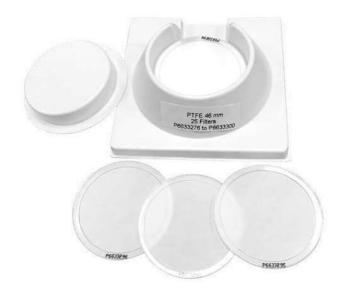
GVS PM 2.5 PTFE Membrane is a high-purity, thin membrane for PM 2.5 ambient air monitoring. Each membrane is sequentially numbered with a chemically resistant polypropylene support ring. The low tare mass allows for accurate gravimetric determinations. No glues or adhesives are used in making the membranes and its stable design eliminates curling, keeping the membrane flat allowing for robot use.
